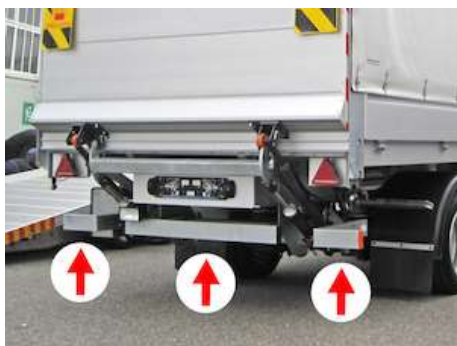
OAF100.ST - Fixed 3-piece bumper STEEL mounted on lift frame
