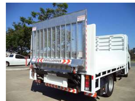
OAP018.01 - Platform DH-LM in meshed steel
