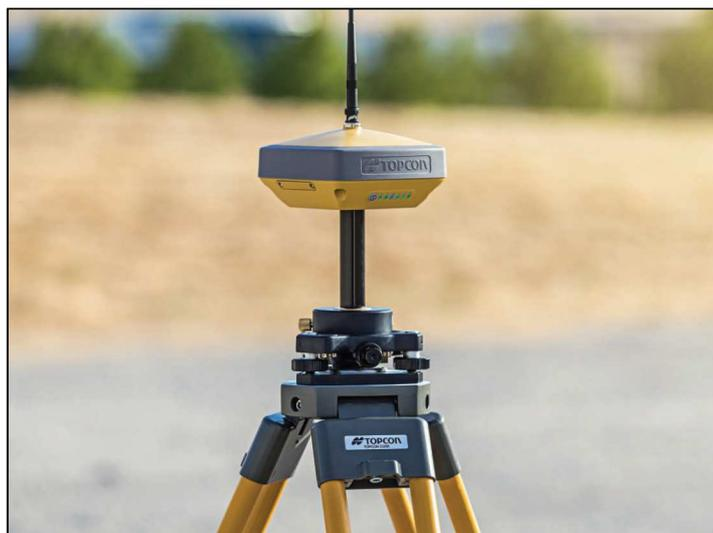
**Figura 3 – Receptor RTK – Topcon Hiper VR**
